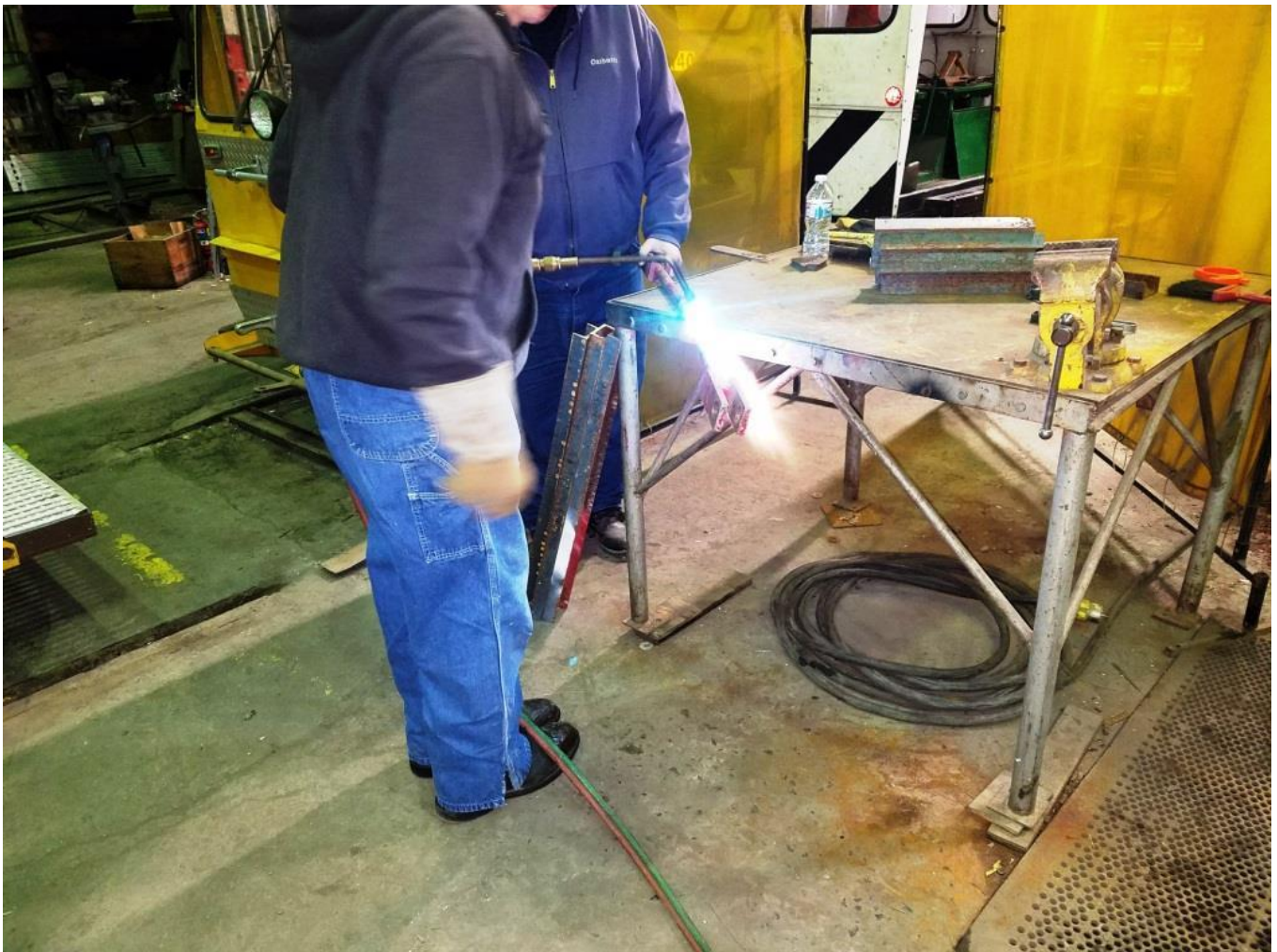
Cliff and Gene heat the bent draw-bar
